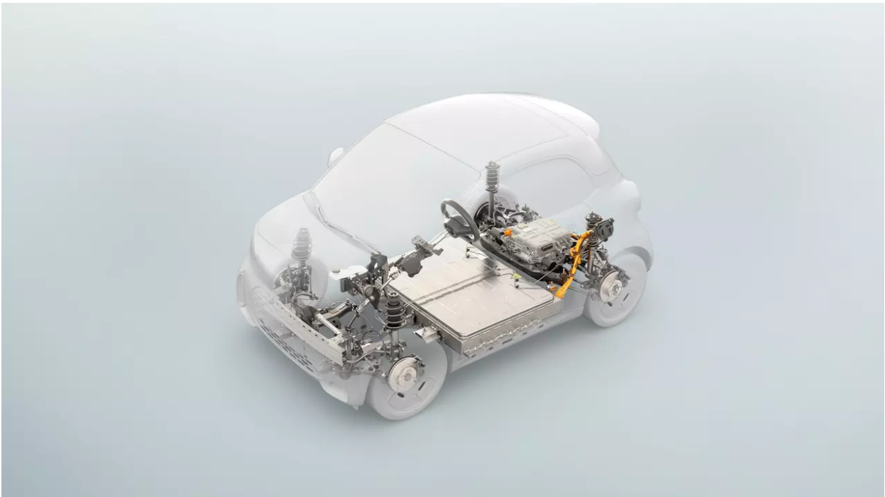
La plateforme Electric Compact Architecture (ECA) de la smart #2
