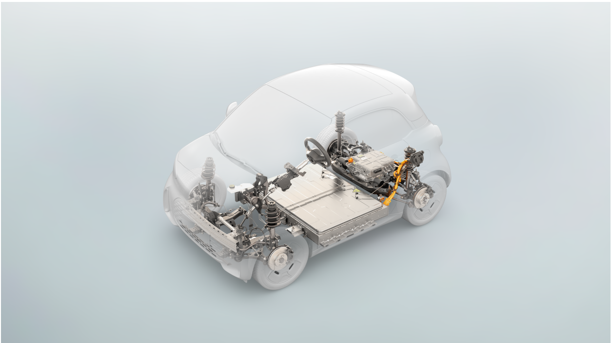
Electric Compact Architecture (ECA)
