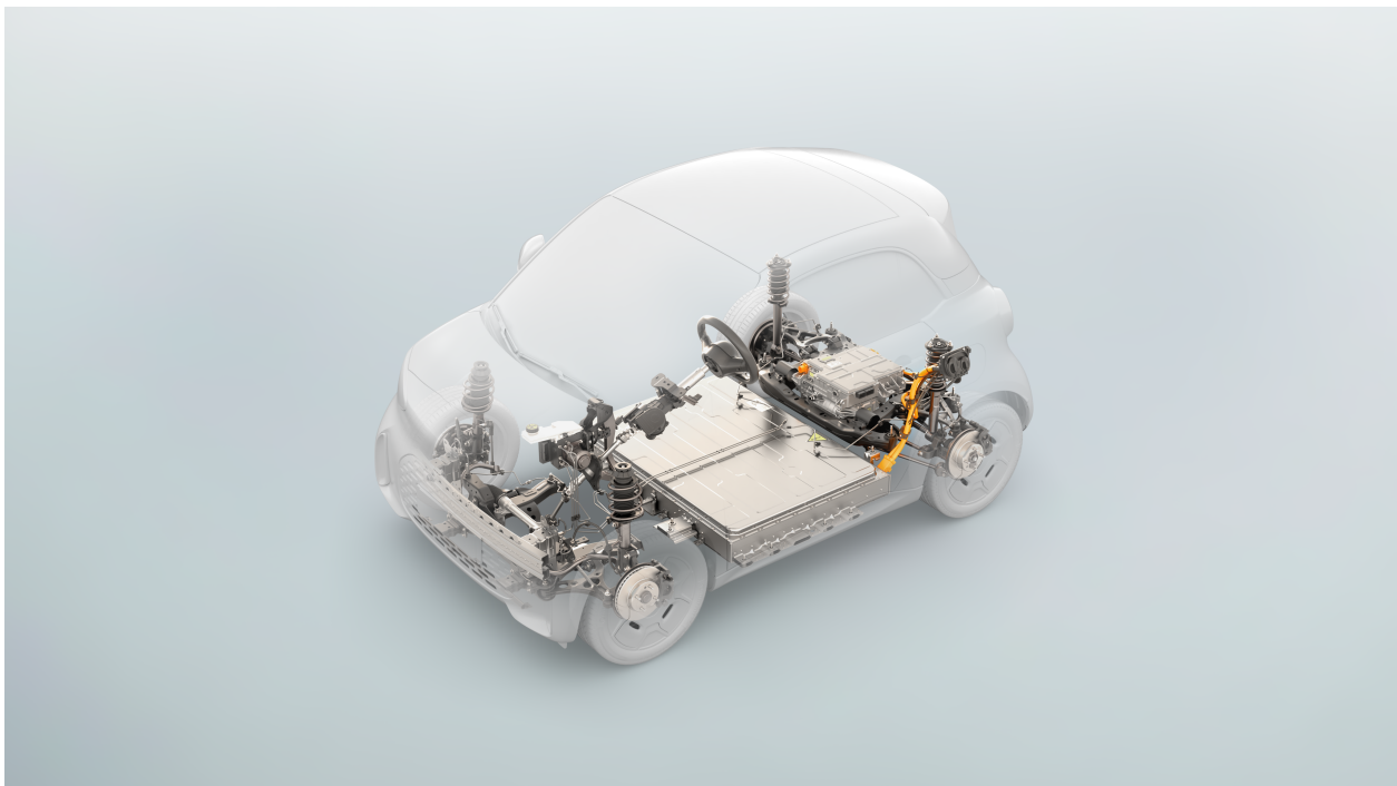
Electric Compact Architecture (ECA)
