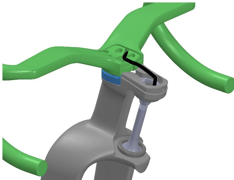
At this point add any spacers in conjunction with the above step, bringing the barstem gradually onto the top of the fork.
