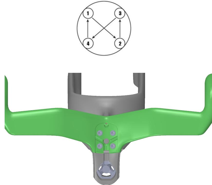
Gradually tighten the bolts in a X sequence, to a maximum of **6 Nm**
