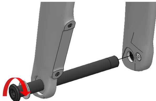
Remove the thru-axle and remove the hub. Install front wheel and tighten the thru axle (with the nylon washer) to **10Nm**.
