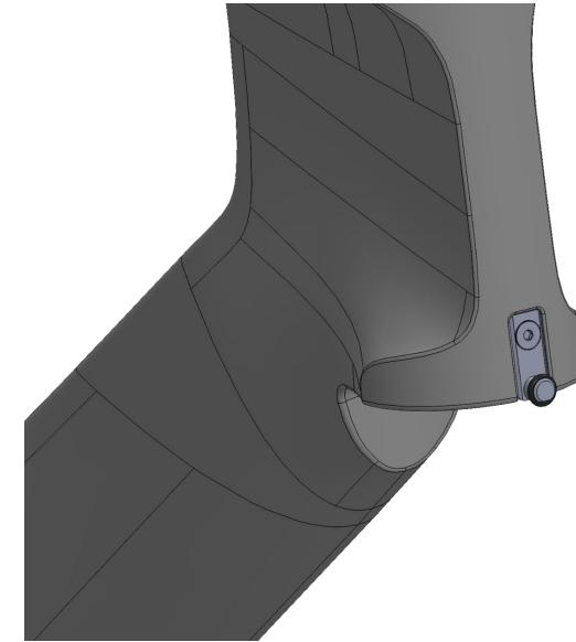
Apply a generous coating of Blue Loc-Tite to the rear of the anti rotation stop, and affix to the frame, torquing to not more than 2-3Nm.
