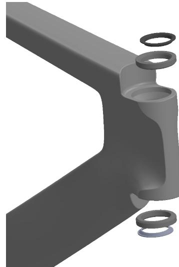
Thoroughly grease the bearing/frame interface, and install the bearings. Use a relatively viscous di-electric grease in this area. Grease and place the upper and lower bearing centering rings, note they are marked clearly as upper or lower.
