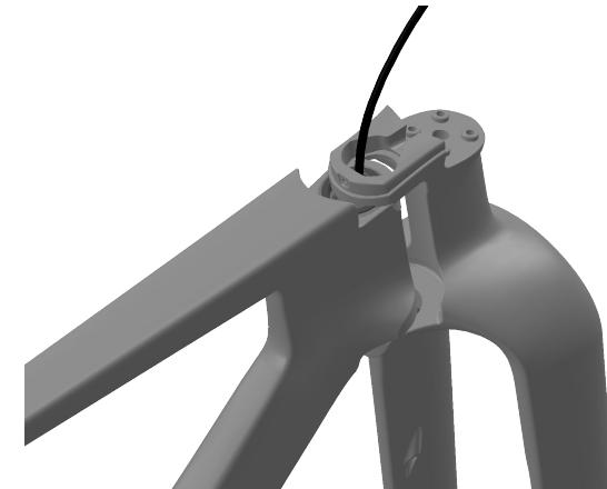
While the grease retains the bearings, slip the fork overtop of the entire head tube assembly. If you have already pulled the hoses through the frame then pull them through, otherwise install the brake hoses after the HS is assembled.
