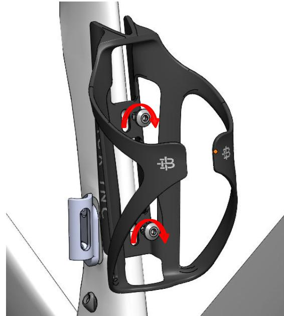
Install cages of your choice and tighten M5 bolts with a high quality 3mm Hex head to **2 Nm**.
