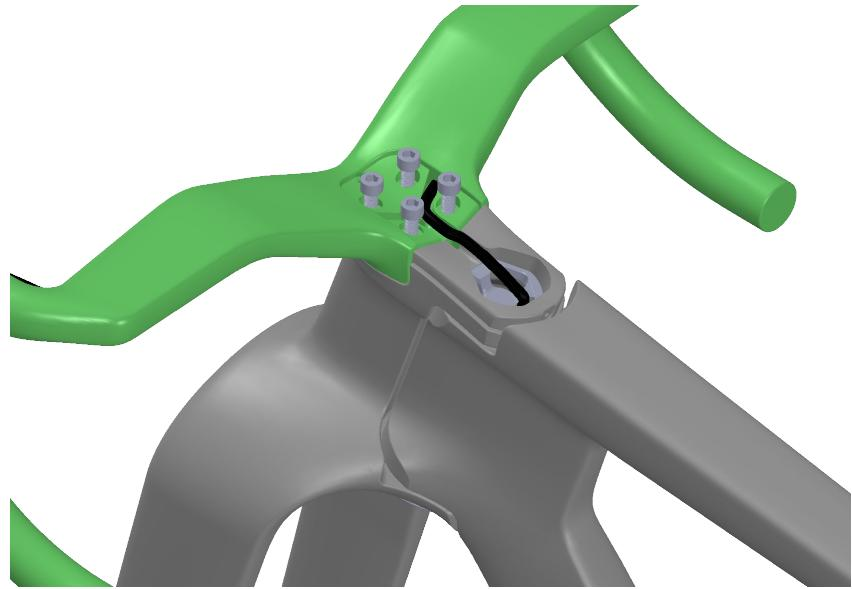
Lightly grease and hand thread in the correct length bolts
