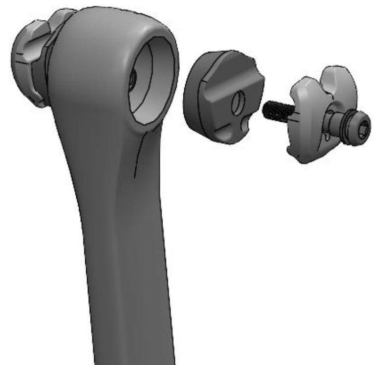
If you are using a 1x setup, remove the FDM and set aside. Install the provided blanking plates for the FD mounting holes. Note you may benefit from a small dab of adhesive or silicone when installing these as they can rattle out with time.
