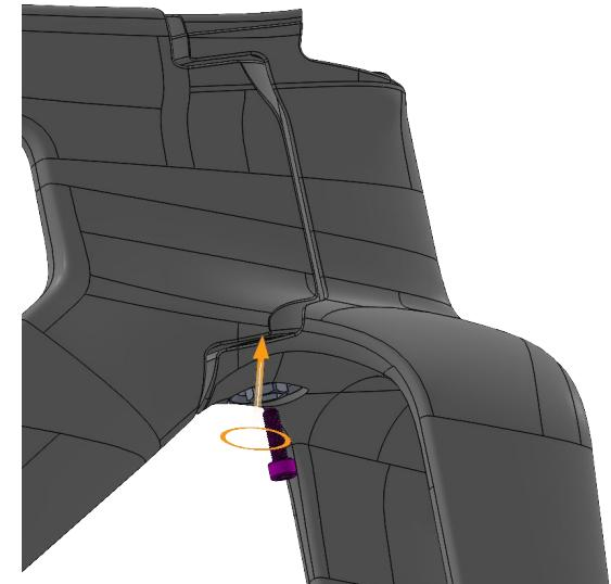
Install and tighten the locking bolt into the preload assembly to lock the collet in place, tighten to 5Nm
