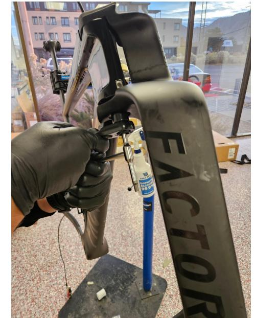
Place the end of a 14mm or passthrough ratchet on the 14mm Collet land. Pass a 6mm allen key through this wrench or socket. Hold the tension rod static with the 6mm Allen while turning and tightening the 14mm ratchet. Tighten to a max of 8Nm, or until snug. Caution must be taken here to not spin the preload rod HS will become over tight.
