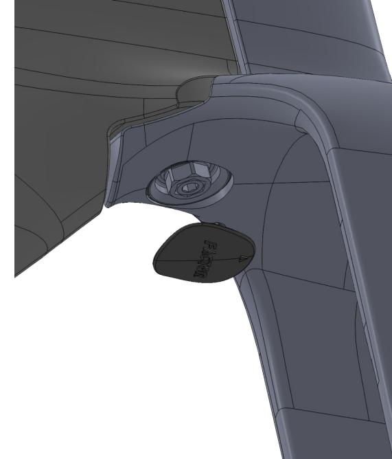
Insert and tighten the setscrew into the underside of the tension rod/collet assembly to lock the collet in place. Ensure the Loc-Tite blue is in place, and add a dab if reinstalling. Install the rubber compression rod protector and ensure a snug fit. If your rider is going to use the bike on rough surfaces such as cobblestones you may want to add dabs of clear silicone to the interfacing surface to add an extra level of security from accidental loss during sustained rattling.
