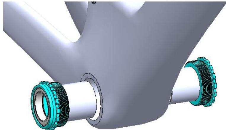
Thread the cups into the frame and torque the cups down to 40nm for both drive side and non drive side. We recommend using the CeramicSpeed T47/T45 Dual Socket Tool.
