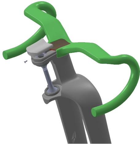
Incline the handlebar to the left or the right, and install the compression cover to no more than 1.5Nm
