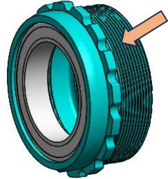
Clean the inside of the frame bottom bracket & the bottom bracket cups with an isopropyl alcohol.
