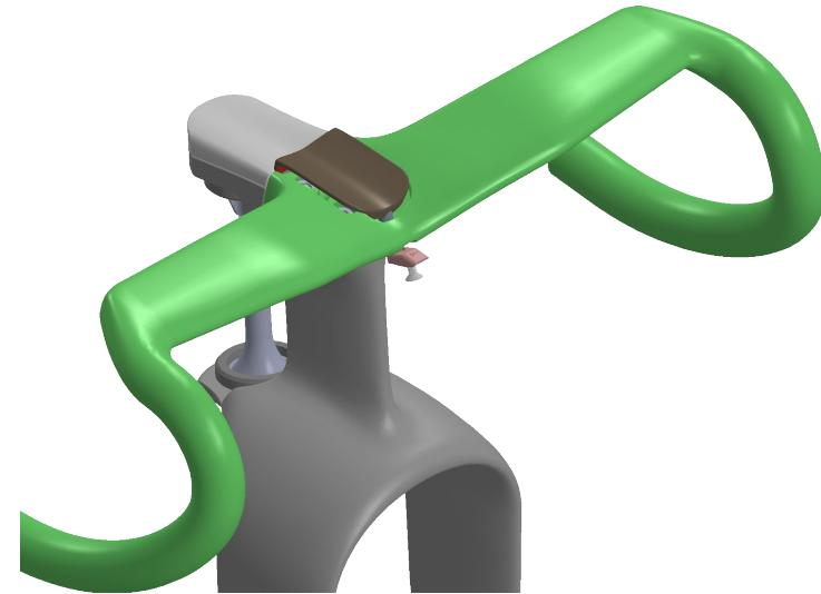
Working from the computer mount, either install the computer mount or the blanking plate followed by the associated screw to affix the barstem cover using a torque value of **2Nm**
