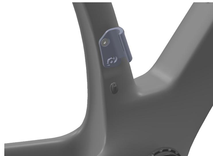
If you are using a 1x setup, remove the FDM and set aside. Install the provided blanking plates for the FD mounting holes. Note you may benefit from a small dab of adhesive or silicone when installing these as they can rattle out with time.
