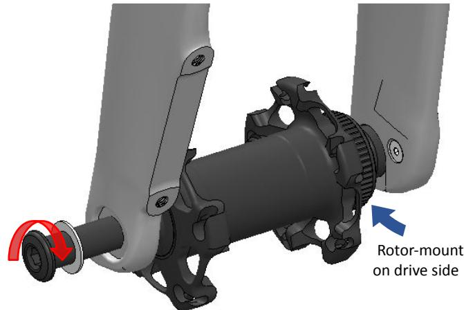
After ensuring the dropout insert is correctly aligned, tighten the dropout bolt to **1 Nm**.
