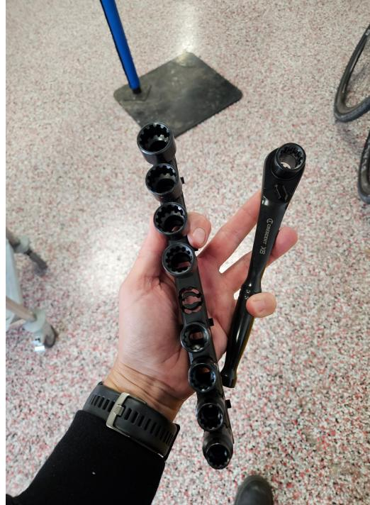
A high quality 14mm pass-through socket is strongly recommended for tightening the collet.
