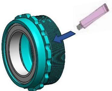
Apply a layer of good quality assembly paste to the threads of both bottom bracket cups. We recommend assembly paste from Morgan Blue (Auqaproof Paste) or r.s.p. (Creak Freak Assembling Paste).
