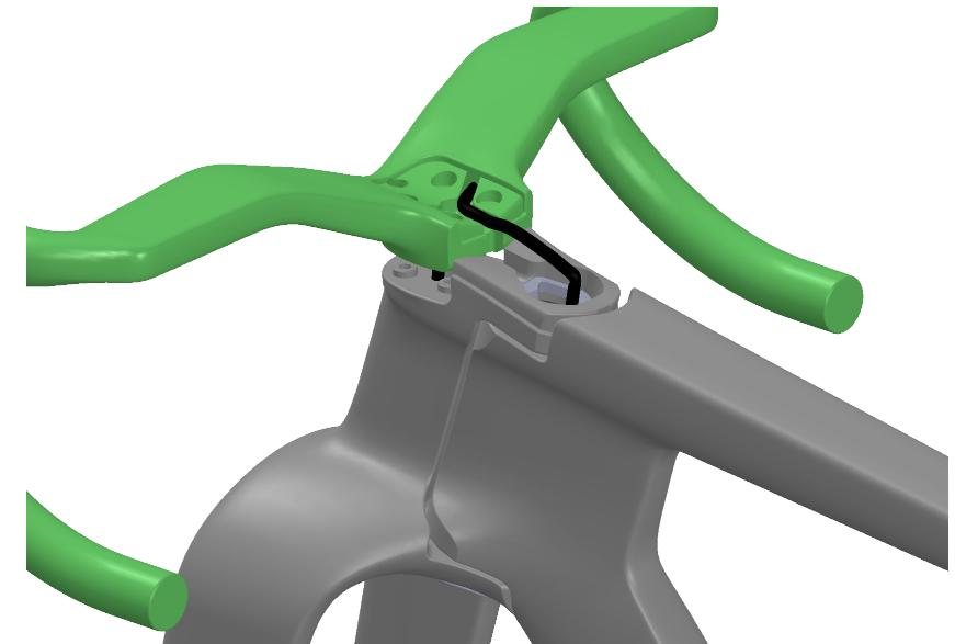
Pull excess hose from the frame through the barstem gently, inching the two components together until snug.
