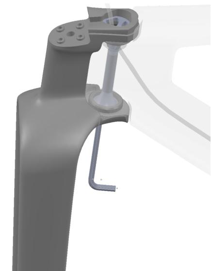
Use an 6mm allen key to tighten the preload until adequate. Its good practice to “overload” the HS somewhat to facilitate the seating of the bearings and centering rings, then back off the preload until the fork turns freely.
