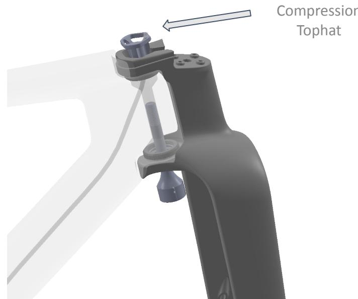
Apply dielectric grease to the outside of all alloy components contacting carbon, hand thread the compression rod to the upper bearing centering compression tophat.
