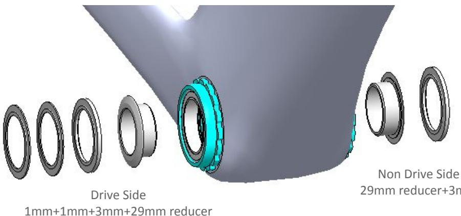
For Shimano Hollowtech II cranksets, install the included 24mm Wheels MFG reducers and spacer in the following sequence.
