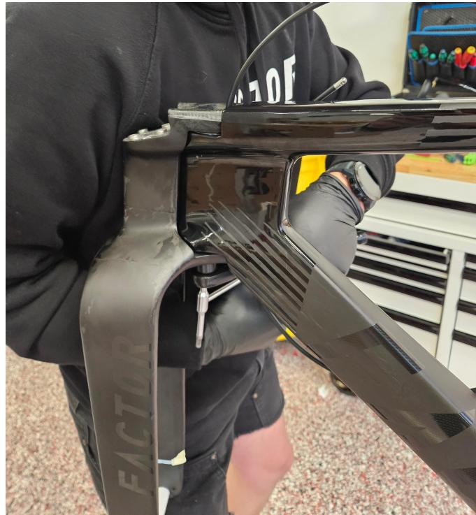
Place the end of a 14mm or passthrough ratchet on the 14mm Collet land. Pass a 6mm allen key through this wrench or socket. Hold the tension rod static with the 6mm Allen while turning and tightening the 14mm ratchet. Tighten to a max of 8Nm, or until snug. Caution must be taken here to not spin the preload rod HS will become over tight. You may find it helpful to brace your arm against the fork to hold the preload rod static.
