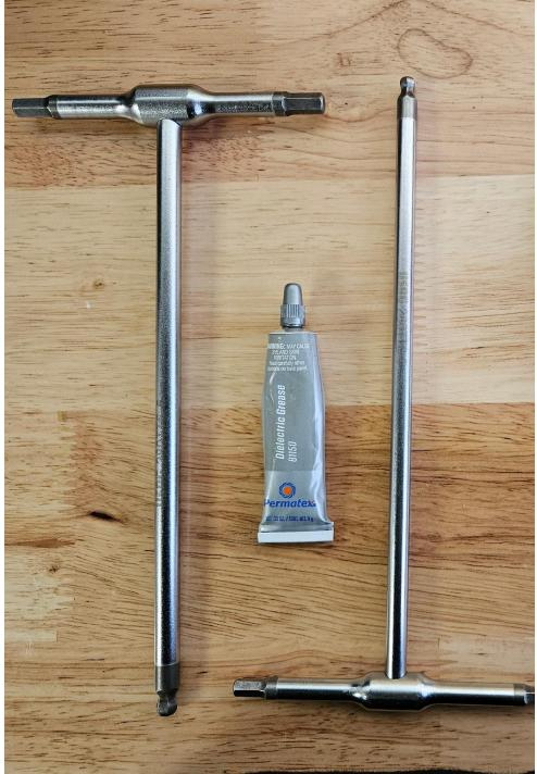
High quality T-Handle hex wrenches (6 and 5mm) are recommended for the next steps. A high quality dielectric grease acts to insulate the aluminium compression rod from the carbon and prevent galvanic corrosion from occurring. Many conventional greases also have dielectric (non-conductive) properties.
