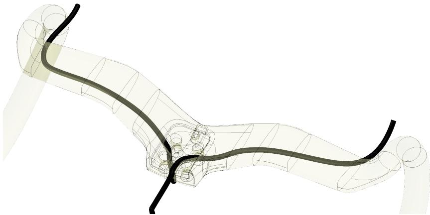
Snake hoses the hoses coming from the top of the frame and fork through the bar, respecting which is left and which is right and corresponding front/rear brakes
