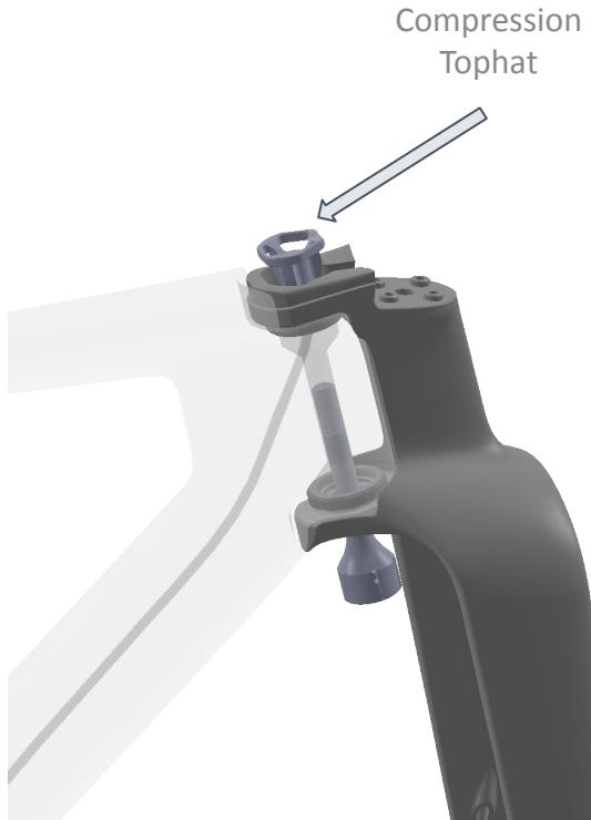
Apply dielectric grease to the outside of all alloy components contacting carbon, hand thread the compression rod to the upper bearing centering compression tophat.
