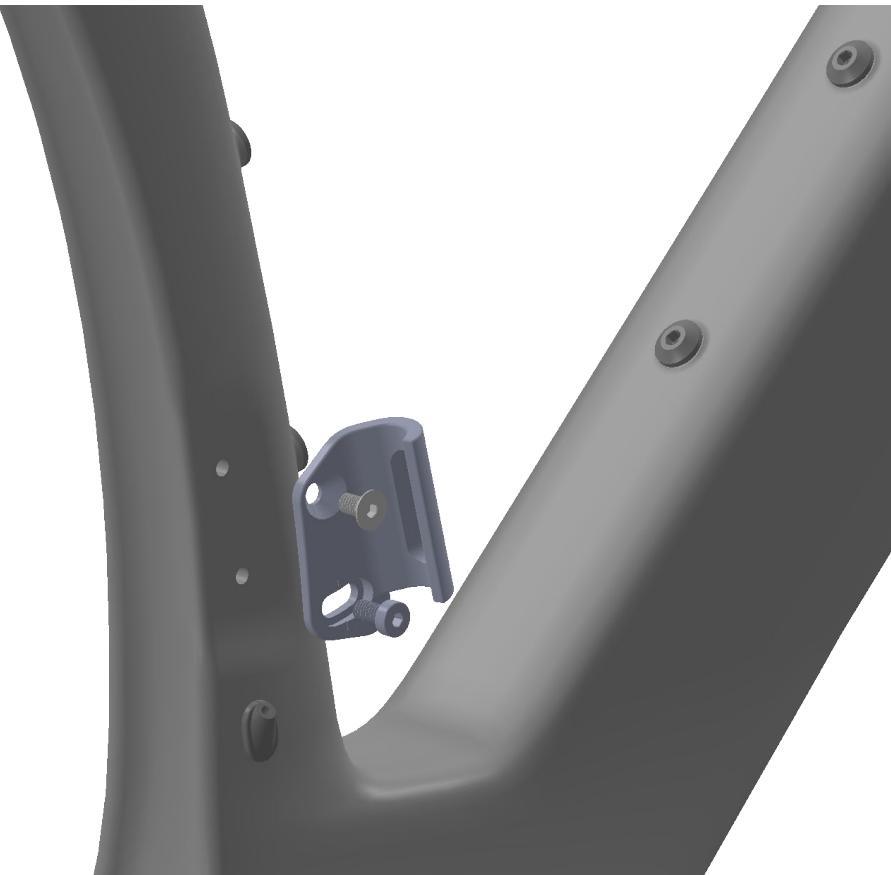
Your frame is provided with blanking plates for wireless shifting, and grommets for shifting needing electric wires. Install both at the FD and the RD to prevent foreign material ingress.
