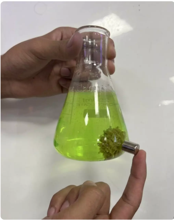
▲ Demonstration - Handheld magnet attracts formed clumps
