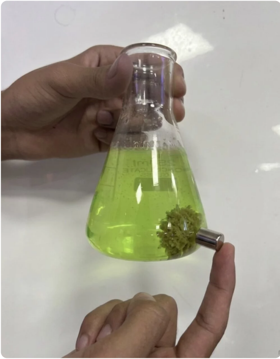
▲ Microplastics removal step 3 demonstration - magnet use
