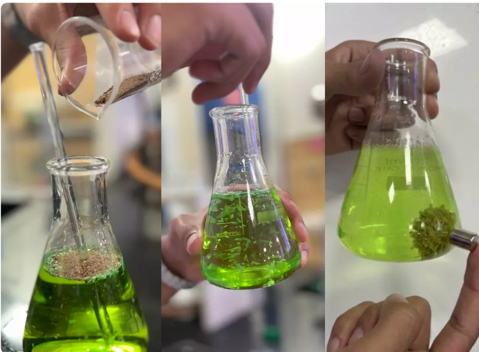
▲ 3-phase demonstration - Adding the powder to coloured water, mixing, and attracting clumped microplastics using a handheld magnet
