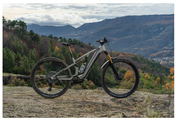
Lightweight, speed and integration are the defining qualities of the new Stereo Hybrid ONE55 C:68X, which makes use of up to six different fibre types to meet the specific demands of each part of the frame. The result is a chassis that's the lightest e-mtb in tube frame we've ever built – up to 20% lighter compared to our Stereo Hybrid 140 frame.
