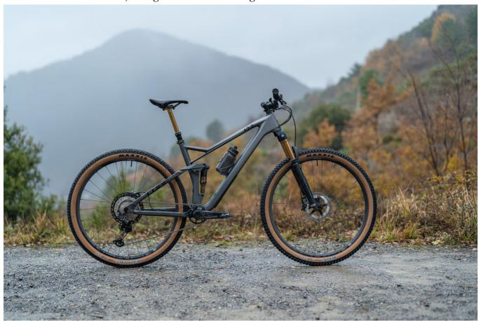
The brand-new Stereo ONE44 promises all-mountain performance, with a choice of advanced C:68X or C:62 carbon frames, 140 mm of progressive travel, adjustable geometry and a built-in storage compartment.
