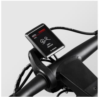
And on the subject of mixed terrain, the ingenious Bosch ABS (Anti-lock Braking System) prevents front wheel skidding and rear wheel lifting if you suddenly need to slam on the brakes.
