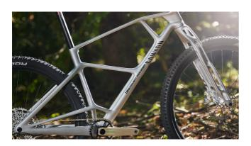
To ensure structural reliability, Thumm and his team used CAD simulation software to study the forces applied during mountain biking. Together with input from engineers and designers, this allowed a very distinctive frame shape to be developed, optimally designed for the stresses of riding. Struts in the frame triangles ensure an ideal force distribution and an asymmetrical rear triangle allows for targeted power distribution with minimal use of materials.
