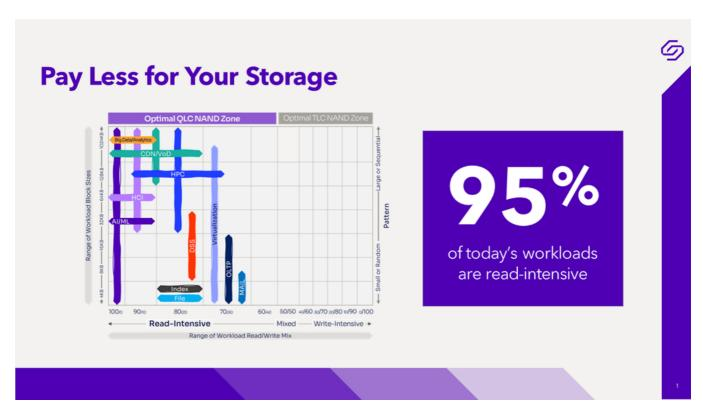
The reason for this right-sizing is that workloads and drive behaviors are better understood now. In the case of SSD endurance, studies with massive sample sizes show that 99% of systems use, at most, 15% of a drive's usable endurance by its end-of-life. [2] Bottom line? QLC SSDs will not wear out as quickly as they once appeared to. And, depending on the workload, you could be overpaying for data storage.
