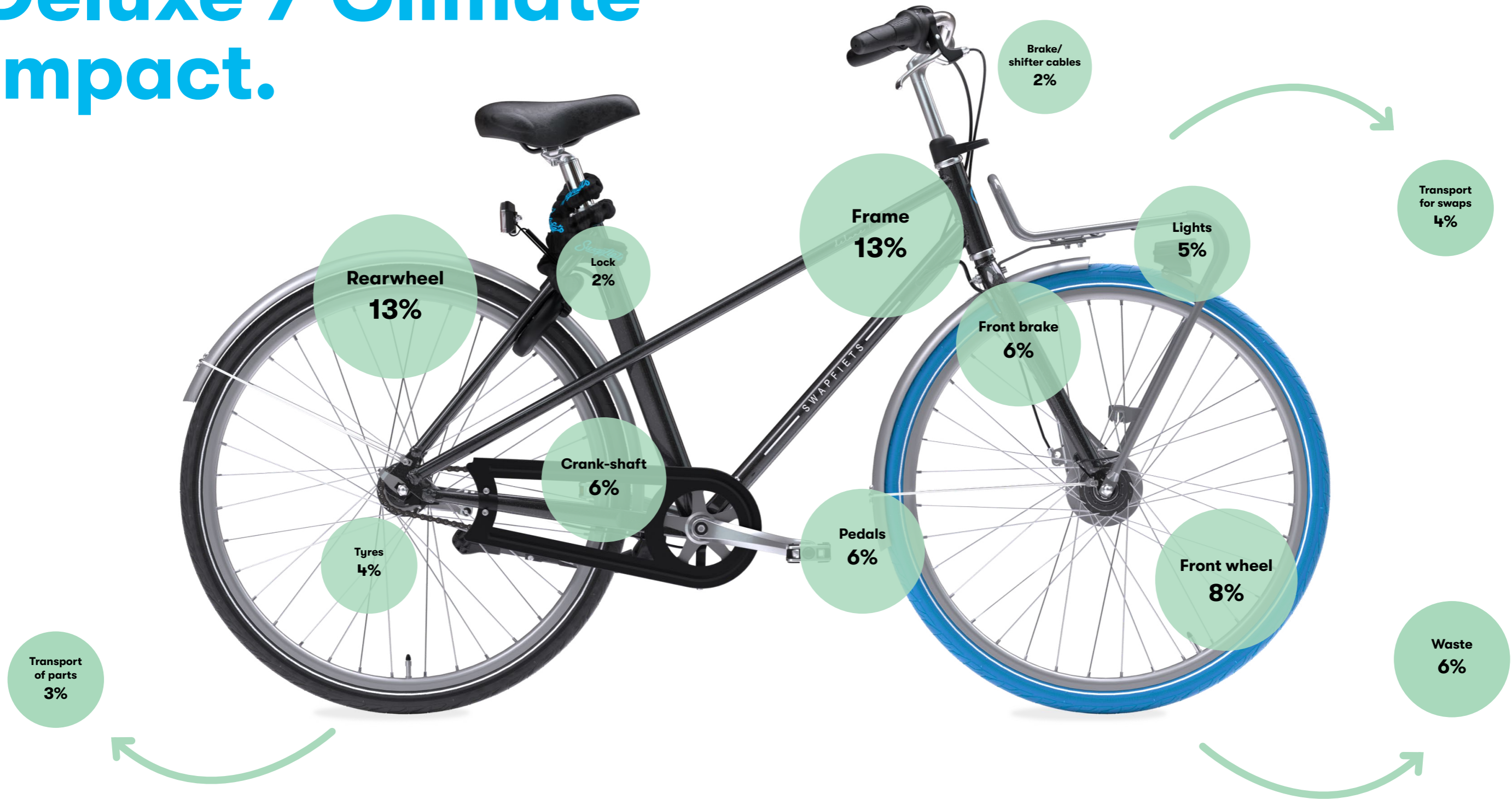
Percentage distribution of global warming impact over processes and top 10 components with the highest impact of the Swapfiets Deluxe 7.
