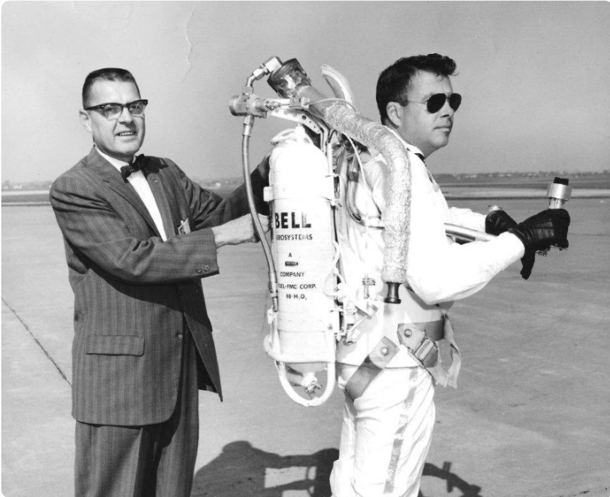
▲ Invented by Wendell Moore, the Bell Rocket Belt Jet Pack took its first flight in 1960.
