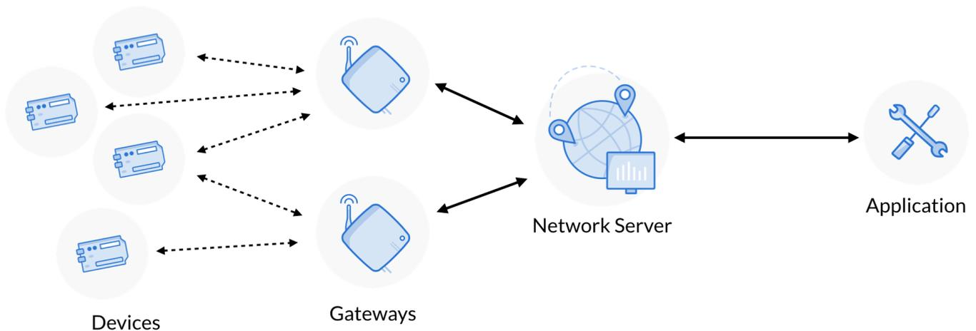
Unlike cellular technology in licensed spectrum, many LoRaWAN networks use overlapping channel plans in the shared spectrum. Since gateways forward all packets, networks receive packets from all devices covered by their gateways, even packets intended for other networks. This gives the LoRaWAN ecosystem the unique opportunity for exchanging traffic between networks: once a packet is received by a gateway, the cost to forward the packet to the device's home network is near zero.
