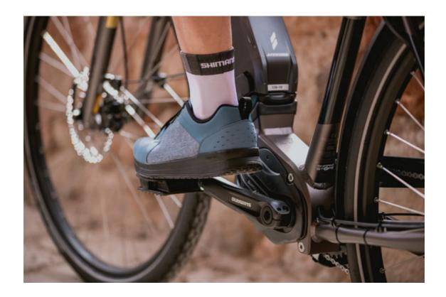
Both pedals have a large concave platform to create a wide contact patch with shoes and to create a stable pedaling platform. The new PD-EF205 has a closed aluminium body with a resin friction plate to create a stable platform for Trekking and Urban riding with formal shoes. On the other hand PD-EF202, with its open muck-shedding design, is intended more for e-MTB usage with casual or sports shoes.
