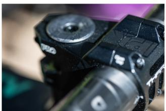
To accommodate the new 35mm beefier clamping area on the bars, a new CNC machined Tharsis stem is also available. This alloy 7050 stem weighs 150g and is available in 35mm, 45mm and 55mm lengths, coming with 0 degrees head angle and a stack height of 4mm.
