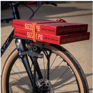
The Pizza Rack comes with everything needed to Eyelet mount the rack on the front of your bike, but it can also be mounted to the axle with various Fit Kits, making it possible to mount the OMM racks to suspension forks, full-suspension mountain bikes, gravel bikes, road bikes, fat bikes and even tri-bikes if that's what you're into.
