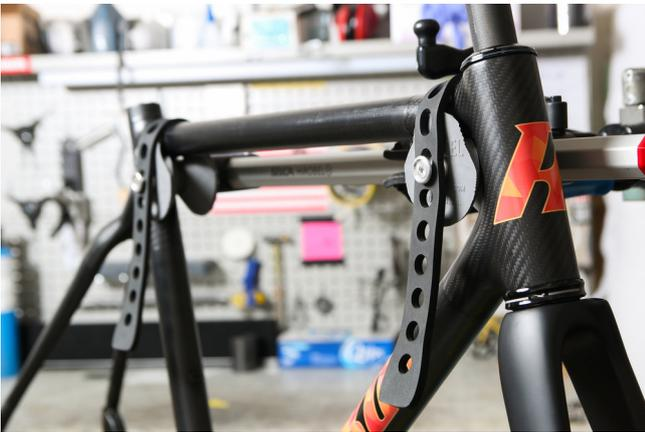
Unique in the cycling industry, the Hirobel is a specially designed repair stand clamp developed for greater compatibility with the needs of today's frames and components. The Hirobel distributes stresses and loads through the bicycle frame rather than just clamping the seatpost or \*gasp\* a frame tube, improving stability while eliminating possible crushing forces.
