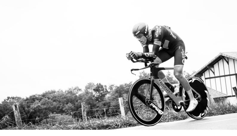
Based on only two carbon spokes with NACA profile and a variable rim height between 48mm and 90mm, all aspects are designed to reduce the drag behind the wheel. From the first tests this wheel showed remarkable improvements compared to the more traditional time trial wheels out there. By using Toray 800 and 1000 UD carbon fibers the stiffness and strength of this wheel are ensured. The materials and shape combined make it a perfect balanced wheel.
